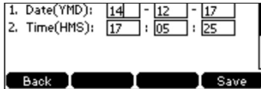
3. Press the **Save** soft key to accept the change. The time and date displayed on the LCD screen will change accordingly.
